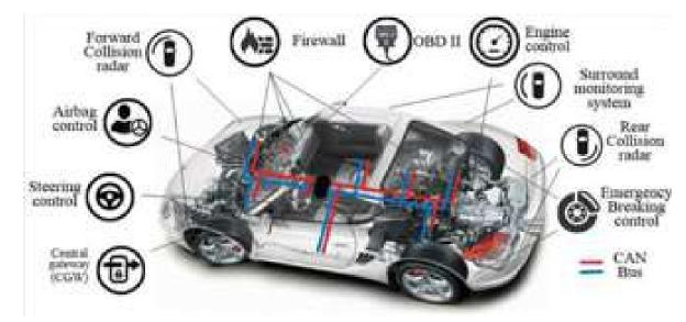
A representation of the architecture of car with a CAN Bus
